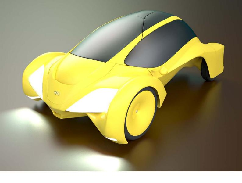
The windows are designed to allow as much light as possible to enter. The use of electrochromic glass gives the possibility of dimming by pressing a powered switch in order to control the level of illumination of the interior.
