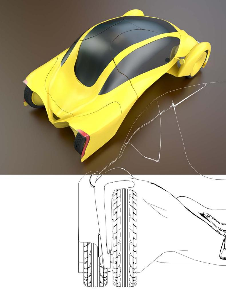
On the back, surfaces curve smoothly into one another and embrace the back wheels, creating a wraparound, retractable trunk that opens like a drawer. Additional security features include smart sensors in the vehicle.
